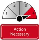
Optimum comfort and health is achieved when relative humidity is maintained between 30% and 55%. Readings outside these boundaries may indicate ventilation issues which contribute to an increase of energy used to condition the space.
